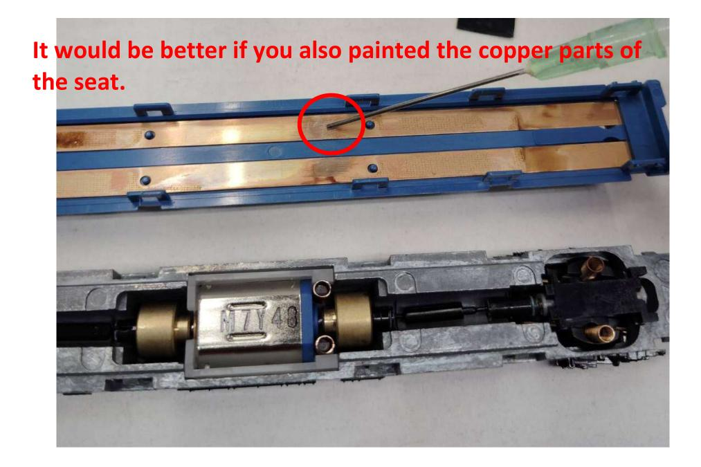
10 Finally, when installing the seat, be careful not to let the powered bogie (shown in a red circle) float. If it does, the seat will not fit neatly.
