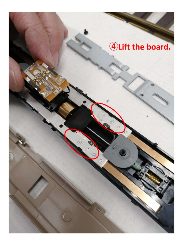
**5** Insert a thin metal plate in the part where the board is lifted (red circle).
