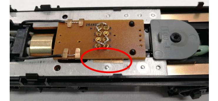
The conclusion is that the contact of the electric transmission is not enough and electricity is not flowing to the motor, so I will energize it by inserting a metal plate.
